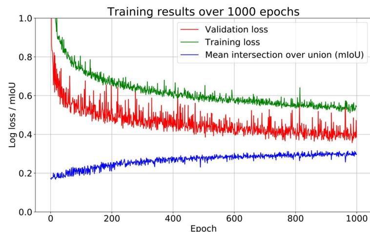
Figure 1. In green and red, the training and validation log loss is compared with mIoU in blue. Over time performance improves with a lower log loss and a higher mIoU.
