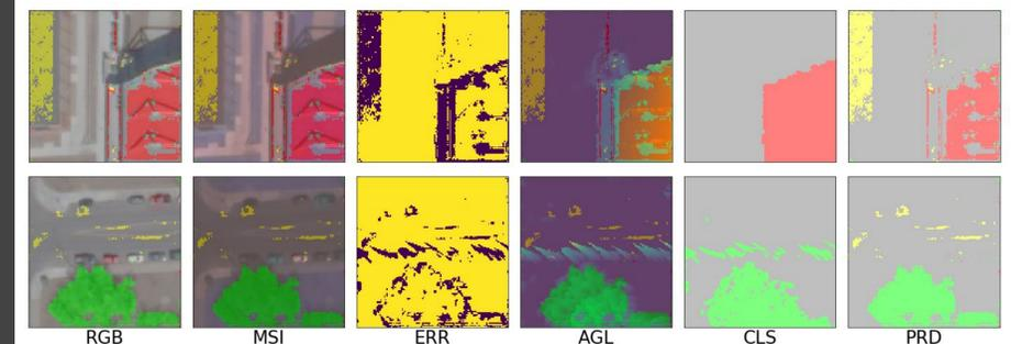
Figure 3. Predictions (PRD) are superimposed on RGB, MSI, and AGL images. Error (ERR) between PRD and ground truth classification (CLS) are shown as purple while yellow represents a correct prediction. For CLS and PRD, red=buildings, grey=ground, green=high vegetation, and yellow=elevated road.
